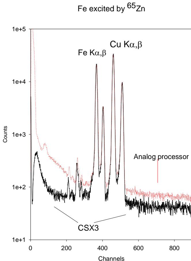
Figure 2. An Fe sample is irradiated with Cu K radiation from a  $^{65}\text{Zn}$  source in transmission geometry, and measured with a Si(Li) detector. The background is substantially reduced using the CSX processors. The manufacturer's analog processor (dotted line), and the Cambridge Scientific CSX digital processor (continuous line).
