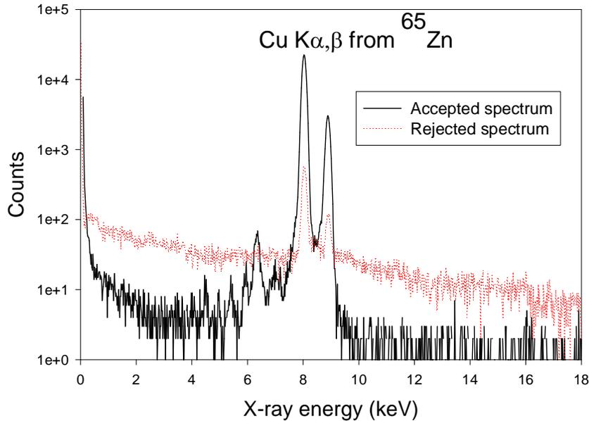
Figure 3. The copper K spectrum from a  $^{65}\text{Zn}$  source measured with CSX3 processor, shows the accepted and rejected spectrum. It demonstrates that the rejected spectrum in this case was mainly nuclear background events. The rejected event spectra of several radionuclides have well defined low energy peaks which merit further investigations.
